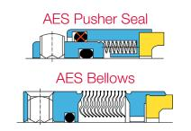
The main advantage of metal bellows seals is the removal of the semi-dynamic sliding elastomer from a pusher seal (shown above with red cross) which removes the potential for mechanical seal hang-up.
