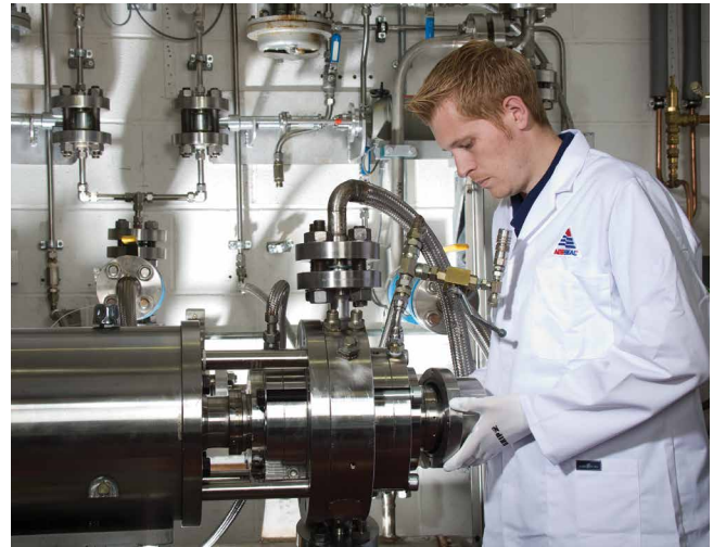
Advanced seal testing on an API 682 specification test rig
