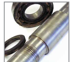
Shaft damage from a labyrinth seal
