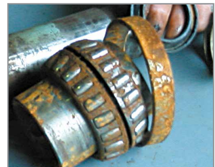
Moisture contaminated bearings
