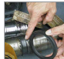
Shaft damage from a lip-seal
