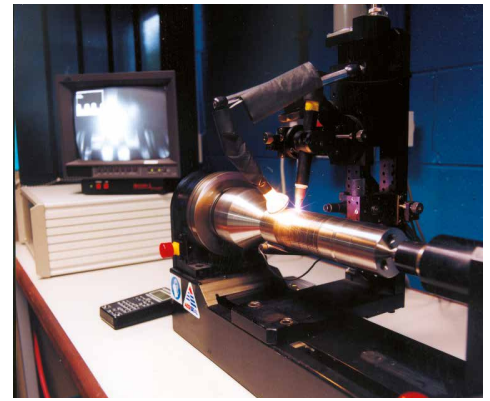
CNC outside diameter bellows welding operation
