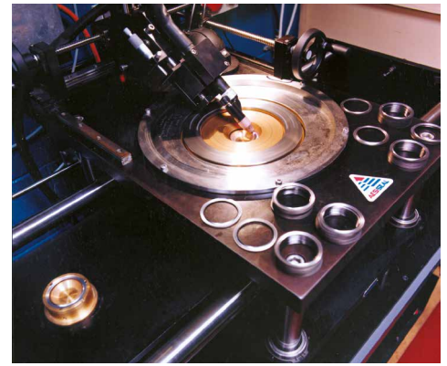
CNC inside diameter bellows welding operation.
