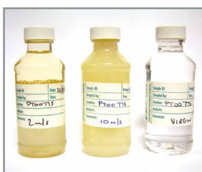
Lip Seal test: Oil sample bottles for laboratory analysis.
