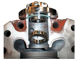
Separate conventional seal and pumping ring configuration.
